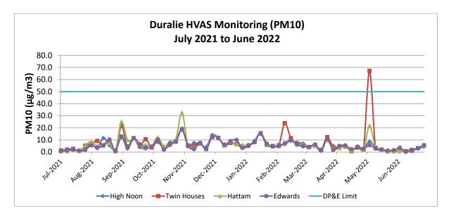
Figure 3-3: High Volume Air Sampling (PM<sub>10</sub>) Results during the Reporting Period
