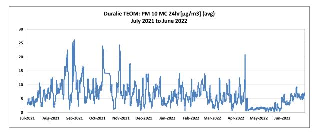
Figure 3-6: Real Time Dust Monitoring (TEOM PM<sub>10</sub>) Results during the Reporting Period
